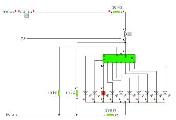
I have now developed it further still so that with a series of clocked input pulses into pin 14 the counter will race through the LEDs, turning them on and off one by one. To select an LED the user has to push and hold down the PTB switch connected to the enable pin.
