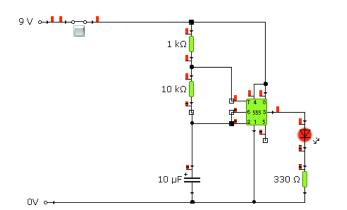
This is another version of the Astable circuit. With the values shown here I have made it give a very rapid train of pulses. By using a potentiometer instead of the 10K resistor I can again make the speed of the output signal variable.
