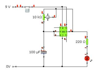
This is a simple Astable or Pulse Generator circuit which gives a series of pulses out of pin3 of the 555IC. The rate of pulses is determined by the values of the 10K potentiometer and the 100µF capacitor.
