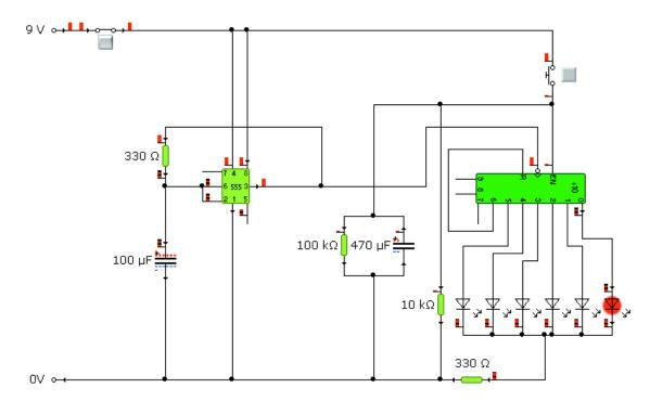
This is my final circuit. With these values this circuit gives approximately 48 pulses per second which is much faster than the eye can see. I can slow this down by increasing the value of the 330R resistor. When the PTM is pressed the decade counter counts through the LEDs for a period of about 7 seconds before selecting one of the LEDs at random. Again I can alter this delay time by varying the value of either the 100K or the 470µF capacitor. **Component calculations on next page**
