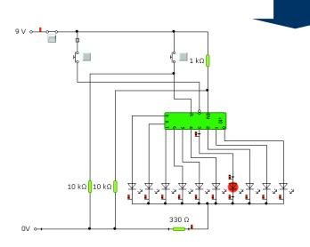
This circuit uses a 4017IC and is a simple counter circuit (which I need for my dice). For every push of the left hand side PTM switch the counter counts on 1 LED.
