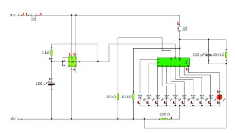
I am nearly there with this circuit. I have now connected my first Astable with the decade counter. It feeds clocked pulses from pin 3 of the 555 into pin 14 of the 4017.
