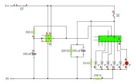
This circuit is almost perfect. It has the 6 LEDs I require but when the decade counter counts up to 6 it then stops.
