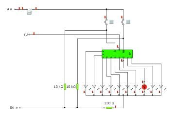
I have now developed the circuit a bit further. With this circuit if I hold down the right hand side PTM switch which is connected to the enable pin, the counter counts through the sequence of LEDs until I let go.
